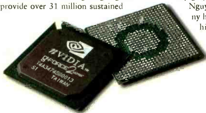
NVIDIA's new tuner chip can translate the 18 ATSC formats and may have applications in computer-centric displays.
